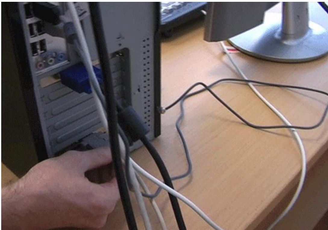
Figure 4 - Attaching the data cable to the computer
