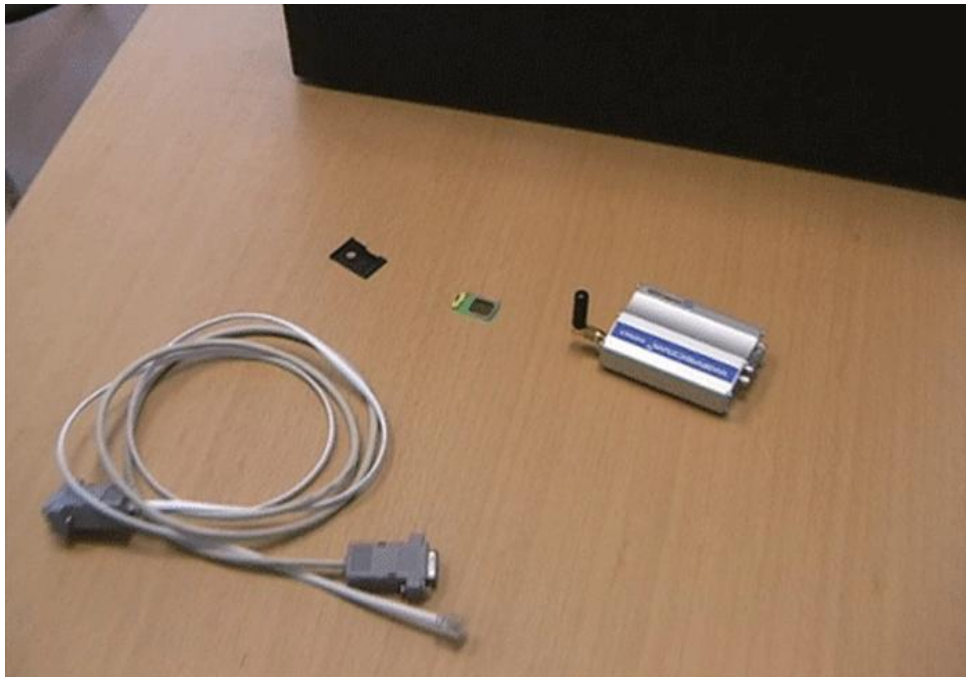
Figure 2 - Wavecom GSM Modem with accessories
